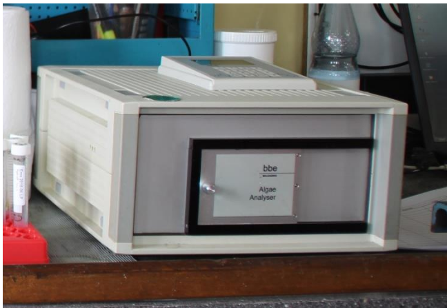
Abb. 4: AlgaeLabAnalyser (Fa. bbe Moldaenke)
